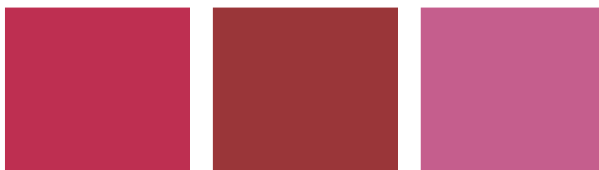
Full shade over white 0.10 % in PVC Full shade over white 0.50 % in PVC White reduction 1/3 ISD in PVC
